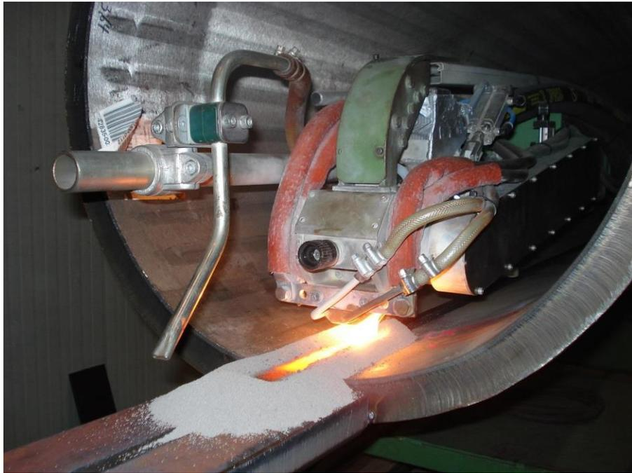
Figure 6: Resistance electroslag (RES) strip cladding of longitudinal DSAW clad pipe
