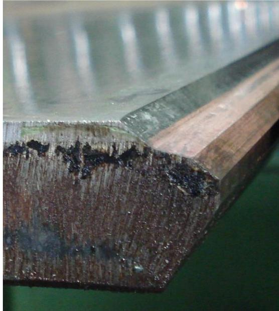
Figure 5: Clad plate with weld bevel preparation
