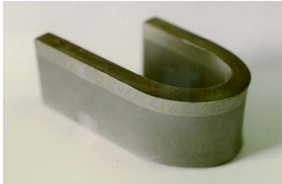
Figure 3: Typical side bend test on explosion clad plate according to ADW8
