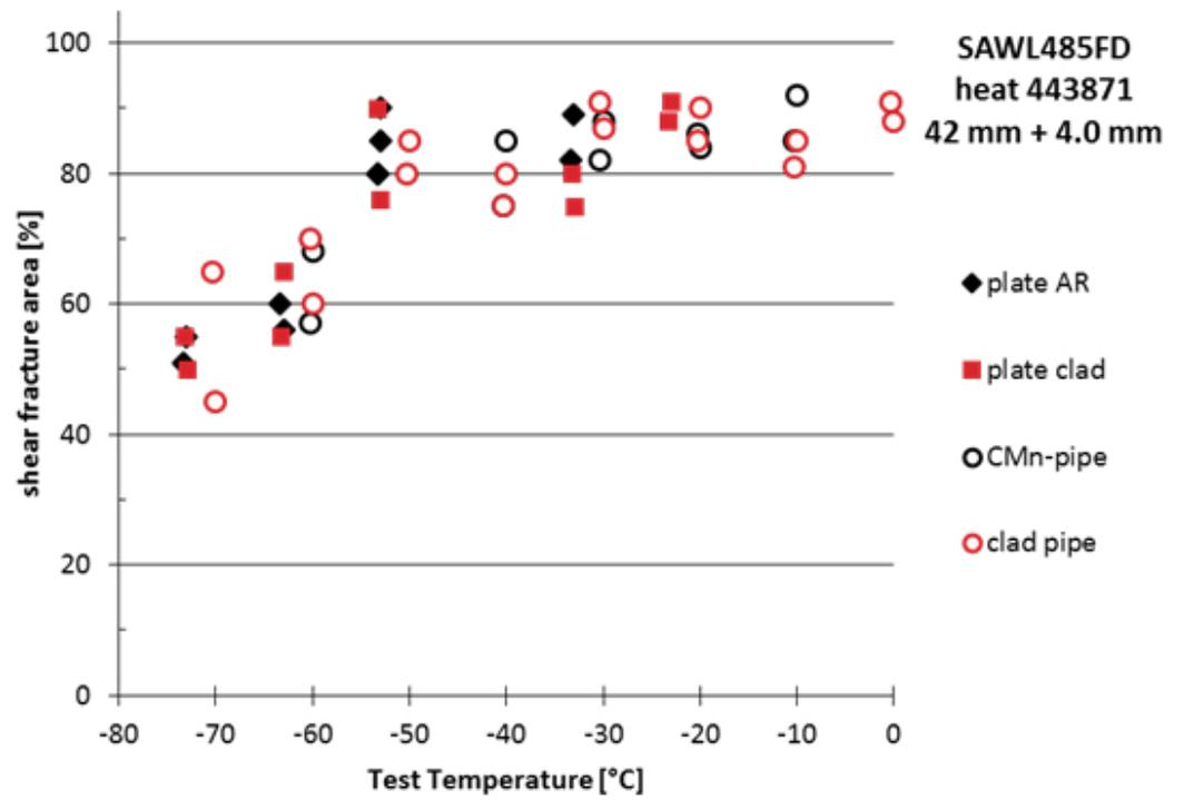
Additionally, the effect of stress relief was not significant for this type of material.
