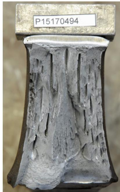
(forming degree 3.9%) seem to scatter a bit more than the plate values, but show, on average, no significant deviation to the plate values. Also similar to the trials #1 and #2 no evidence was found that the explosion welding process alters the brittle fracture control. It is worth noting that the specimens, even at relatively high testing temperatures, show inverse or abnormal fracture appearance. Figure 6 gives an example.
