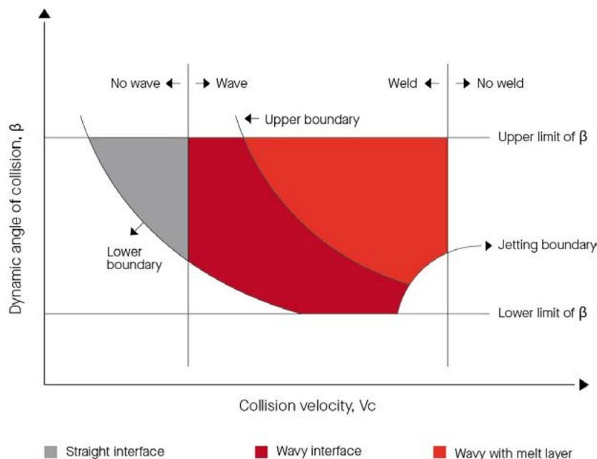
Figure 1: Typical presentation of the Explosive Cladding Window
